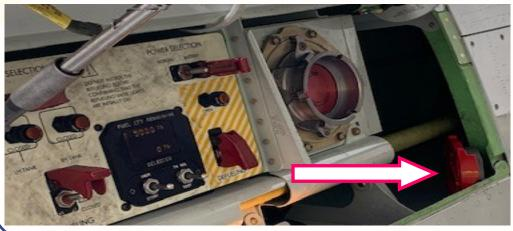
As a reminder, do not place the 175 fuel cap next to the fuel panel when not attached by a chain. The cap could fall back into the wing and cause damage to the aircraft leaving your company responsible for repairs. Notify the flight crew if cap is not attached with a chain.
